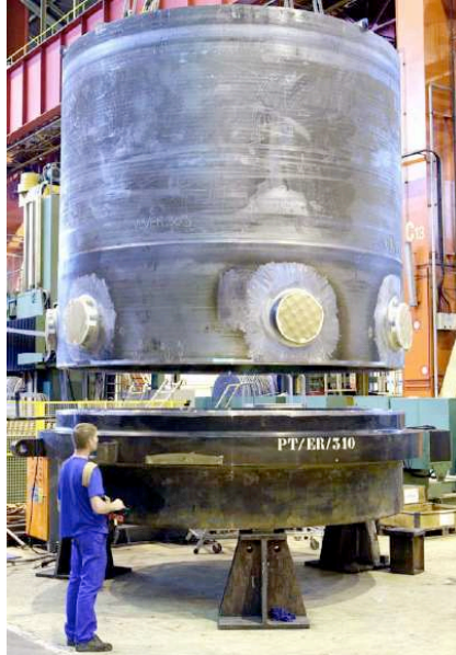
Figure 12 - Large Reactor Pressure Vessel (RPV) forgings with nozzles. (Courtesy of AREVA NP).
