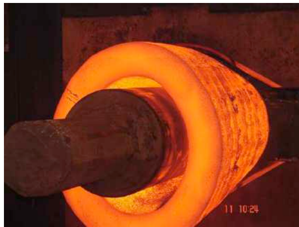
Figure 11 - Reactor Pressure Vessel (RPV) forging. (Courtesy of AREVA NP).
